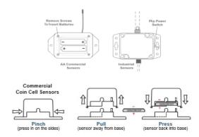
Note: It will take 10 - 20 seconds for the sensor to power up. Configurations for your sensors can be changed in iMonnit. Your new modifications will take effect on the next heartbeat. More immediate results can be achieved by power cycling the sensor. Power cycling is accomplished by removing then re-inserting batteries or using the power switch to cycle the power.
