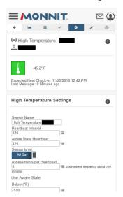
The sensor edit panel allows you to set the primary configurations for the sensor. When you have finished making changed, press the "Save" button at the bottom of this section.
