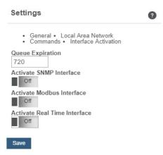
Interface Activation is where SNMP, Modbus, and Real Time TCP Interfaces can be activated. Upon activation, settlings for these will appear in the above menu. Multiple interfaces can be active at one time. All interfaces require the DHCP to set to a static IP address.
